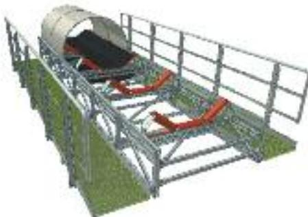
The belt construction is securely braced by telescopic supports. The modular design, which is implemented consistently here too, and the ease of adjustments ensure flexibility and a problem-free execution of the installation.
